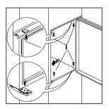
Open the door and push the appliance against the side of kitchen furniture opposite to that of the appliance hinges. Fasten the appliance with 4 screws (I) provided in the kit included with the appliance.
